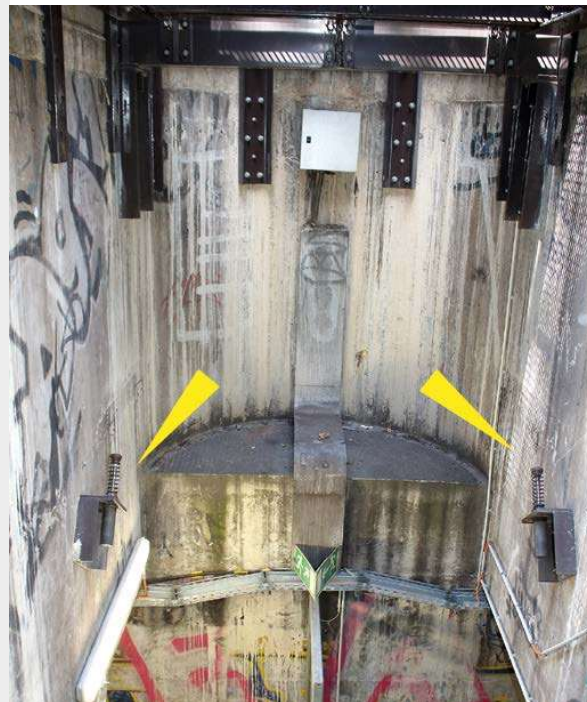
A heavy, five-ton barrier safely stopped by MAGNUM shock absorbers J.P. van Eesteren B.V., 1006 BD Amsterdam, Netherlands
