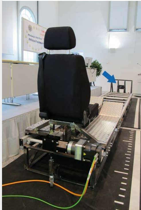
MAGNUM dampers ensure the reliable braking of moving masses on the seat and the protection of the entire carriage construction Central Hessian Police Department, Karl-Glückner-Strasse 2, 35394 Gießen, Germany
